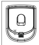
rotate the receiver suspension tab 180° according to the picture; this tab will hold the receiver when used in a suspended position
