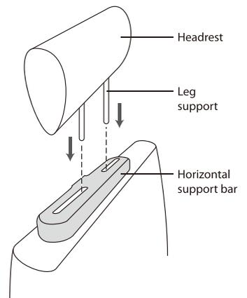
Remark: If the legs of the headrest are too thick for the opening of the horizontal support bar of the bracket, please unscrew the 4 screws of the support bar of the bracket to adjust the opening. In case the screws are too short, use the longer screws (provided in the giftbox).
