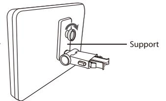
2. Lift the headrest off its leg supports. Align the horizontal support with the headrest leg slots and ensure the horizontal support rests securely on the top of the car seat. Reattach the headrest.
