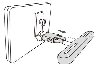
4. Adjust the angle of the DVD unit, then secure by tightening the bolt on the right.
