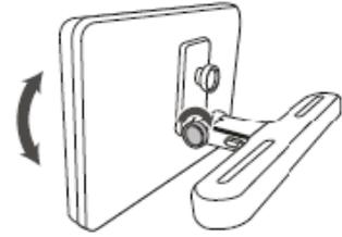
5. To remove the DVD from the horizontal supportbar, support the DVD unit with one hand. With the other hand, firmly squeeze the release buttons on either side of the angled support and pull.
