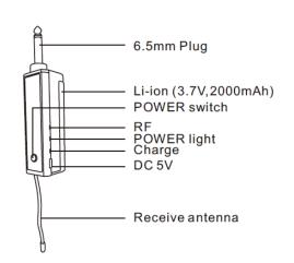
Charge instructions: Charge the receiver for around 5 hours. During charge the LED is green; When fully charge, the LED is off
