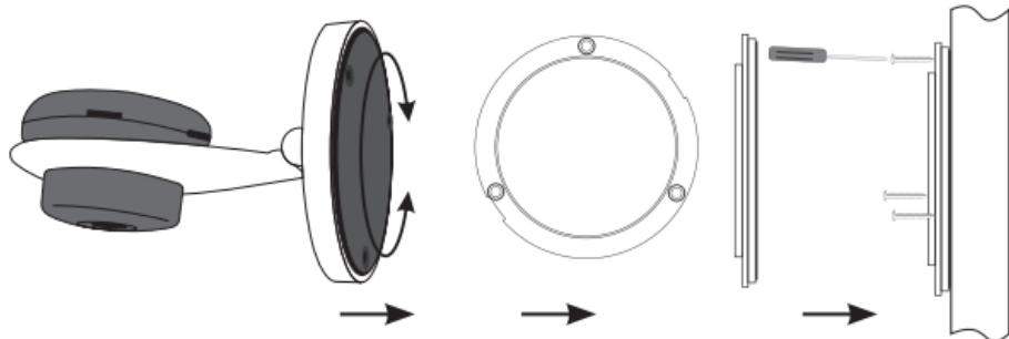
The camera lens can be rotated to straighten up the image.
