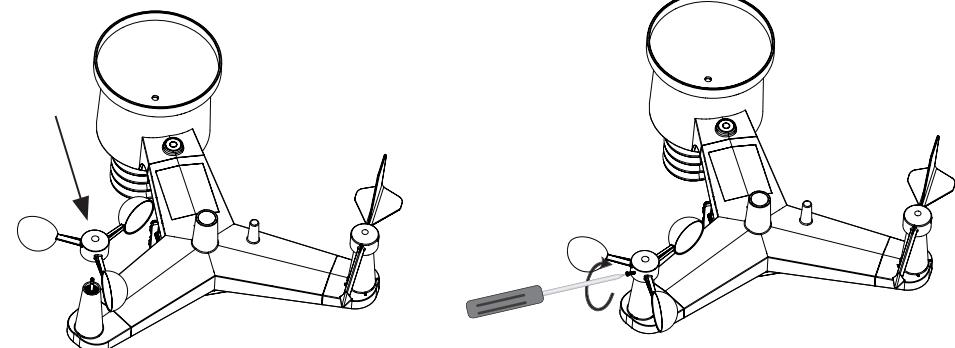
First check whether the small screw of the wind catcher is rotated outward far enough and then push the wind catcher over the axle on the outdoor unit. Adequately push in the wind catcher, but never force it!
