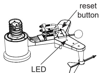
Check whether the indoor unit starts showing values at 'OUTDOOR', blow against the wind catchers of the outdoor unit, pour some water into the rain gauge and check whether the values indicated by the indoor unit change.
