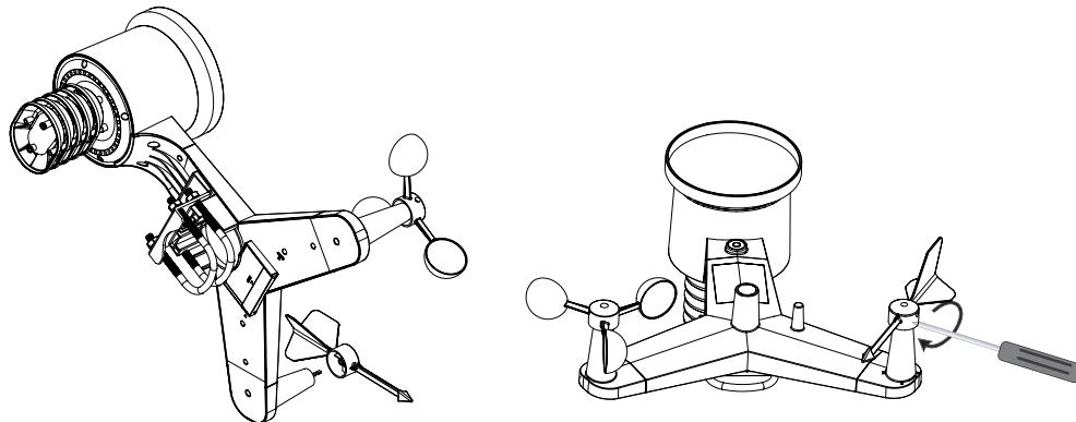
Attention: Both the axle for the weather vane and the weather vane itself are flattened at one end. This ensures that the vane can slide over the axle in only one way. Please keep this in mind during the installation.
