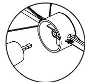
First check whether the small screw of the weather vane is rotated outward far enough and then push the vane over the axle on the outdoor unit. Pay attention to the flattened side!
