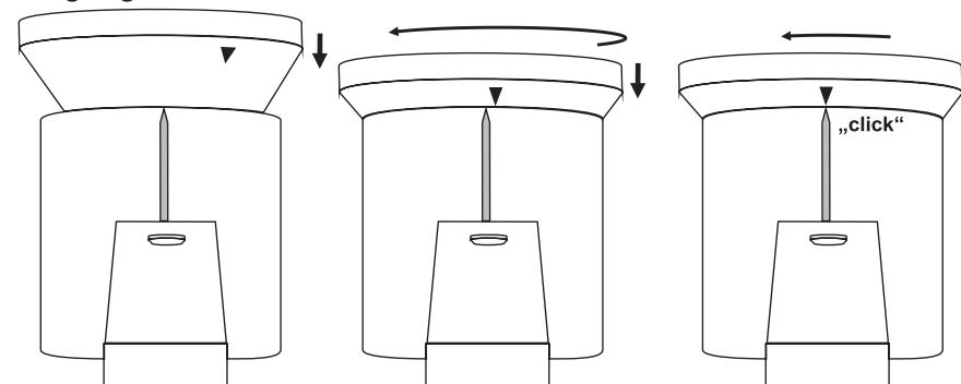
The black rain collection tray must first be placed on the rain unit. There are three markings on the rain collection tray.
