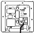
The bottom of the phone is provided with a 'Vibrat' connection for connecting a shaker that vibrates when receiving incoming calls. This shaker is not included, but can be purchased from the Fysic customer service. See the back of this manual for address information.
