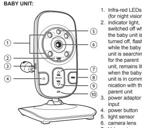
(for night vision) 2. indicator light, switched off when the baby unit is turned off, flashes while the baby unit is searching for the parent unit, remains lit when the baby
