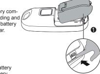
2. Connect the battery plug in the battery compartment according to the figure below and install the battery.
