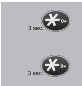
press and hold the \* (asterisk) button for 3 seconds to lock the keypad
