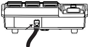
1. plug the telephone wire into the bottom of the telephone
