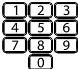
press the desired memory button (0 ~ 9) to dial the corresponding memory number
