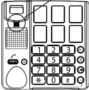
3. slide the receiver clamp out of the telephone, turn it 180° and place it back onto the telephone; this clamp will hold the receiver in case of wall-mounting
