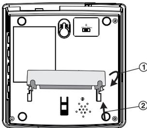
1. click the wall bracket onto the bottom of the phone (1) and press it upward (2) according to the illustration below
