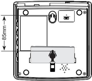
2. in a vertical line, drill 2 holes at a distance of 8.5 cm from each other and insert plugs and screws; let the head of the screws protrude for 5 mm
