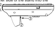
When you want to detach the stand again, press at 3 and remove in the direction of 4.
