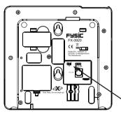
The bottom of the telephone is provided with a small switch for setting the duration of the interruption.
